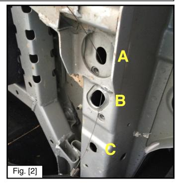
**Step 3.** Attach (1) 7/16"-14x2" bolt, (1) 7/16" inner tooth lock washer, (1) 1/2"D 1"x1-3/4" Plate Washer to the bolt fisher coil and pull the hardware into position in Hole A. Repeat process by feeding coil end of the 7/16" bolt fisher through Hole C and out of Hole B. Repeat for driver side. Step 4 will be complete when 7/16" hardware has been fished into Hole A and Hole C on passenger and driver sides.
